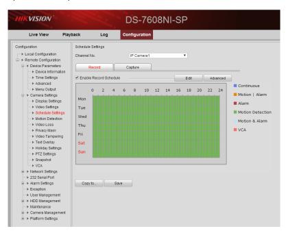
6: Within this section you will see an "Advanced" tab, Click on this and tick the "Enable ANR" box, continue to setup the Pre and Post record times and the stream required.
