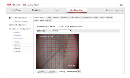
3: Within the Linkage Method at the bottom of the "Motion Detection" page ensure you check the "Notify Surveillance Centre" and "Trigger Channel" boxes. Without this the data recorded while offline will not transfer to the NVR once connect is re-established.
