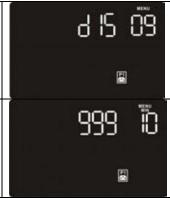
**Step 5:** Press "Up" button (ON/MUTE) to switch to "00" of program list. Then press "Enter" button to exit setting menu.
