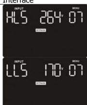
Parameter 1 & 2: Set the acceptable high voltage point and acceptable low voltage point for Bypass mode by pressing the Down key or Up key.
