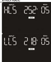
Parameter 1 & 2: Set the acceptable high voltage point and low voltage point for ECO mode by pressing Down key or Up key.
