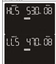
Parameter 1 & 2:Set the acceptable high frequency point and acceptable low frequency point for Bypass mode by pressing the Down key or Up key.
